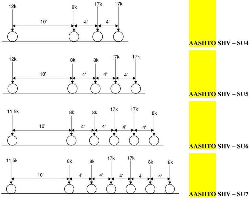
Figure 6.5-2a. AASHTO Short Haul Vehicles (Showing Axle Loads)
