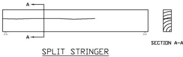
Figure 13.2-1. Cracked, Broken and Split Timber Stringer Defects
